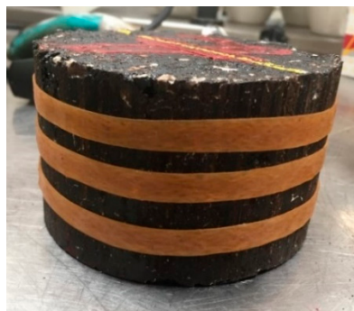
Figure 6. Simulation of in situ confining conditions of the asphalt pavements.
