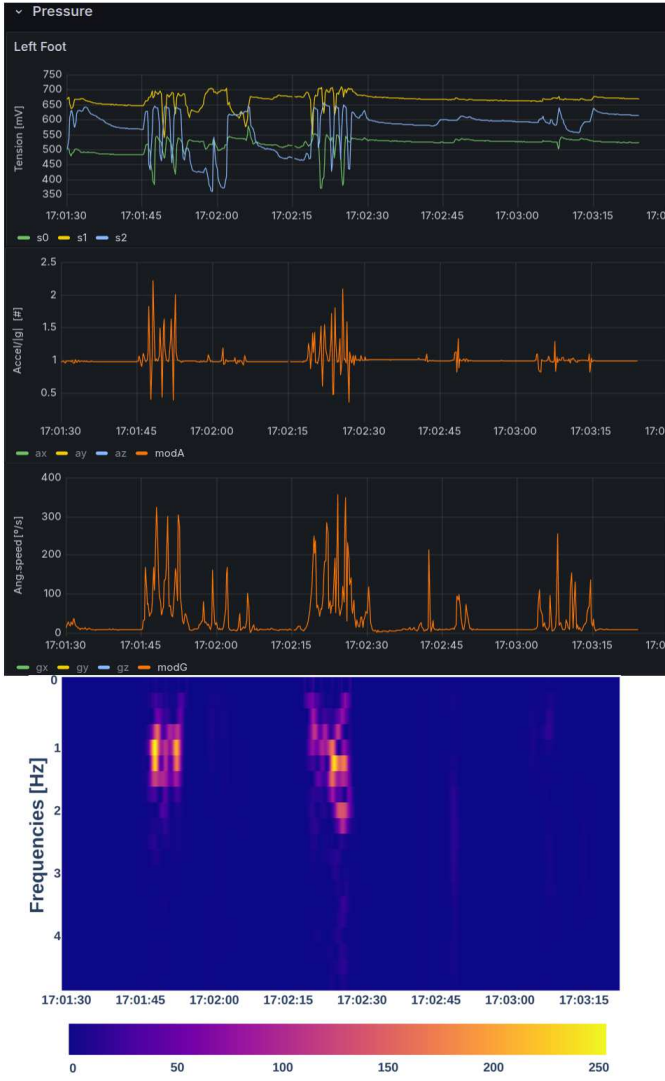
Fig. 6. Spectrogram analysis of walking sequence, where energy concentration near 1 Hz confirms automatic gait detection. This illustrates how frequency-based analysis outperforms simple step counts.
