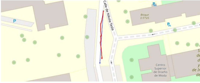
Fig. 5. Trajectory comparison showing that sensor fusion eliminates IMU drift and smooths GPS noise. This demonstrates the reliability of our fusion approach for clinical mobility tracking.
