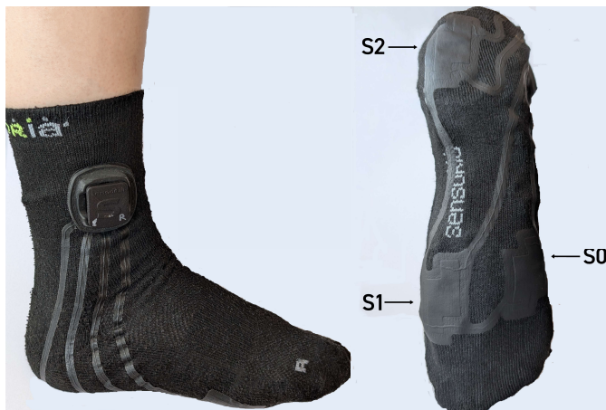
Fig. 1. Sensoria Inc. smart socks with IMU and three pressure sensors per foot (S0–S2), used as the main wearable platform.
