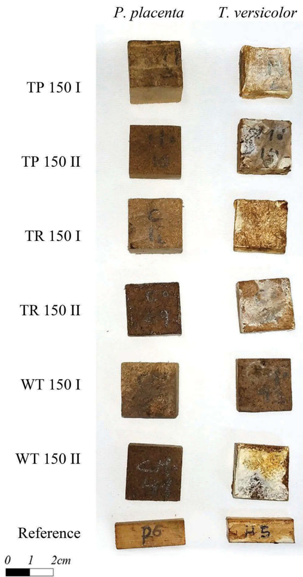
Figure 4. Binderless totora boards and wood reference samples after fungi attack.
