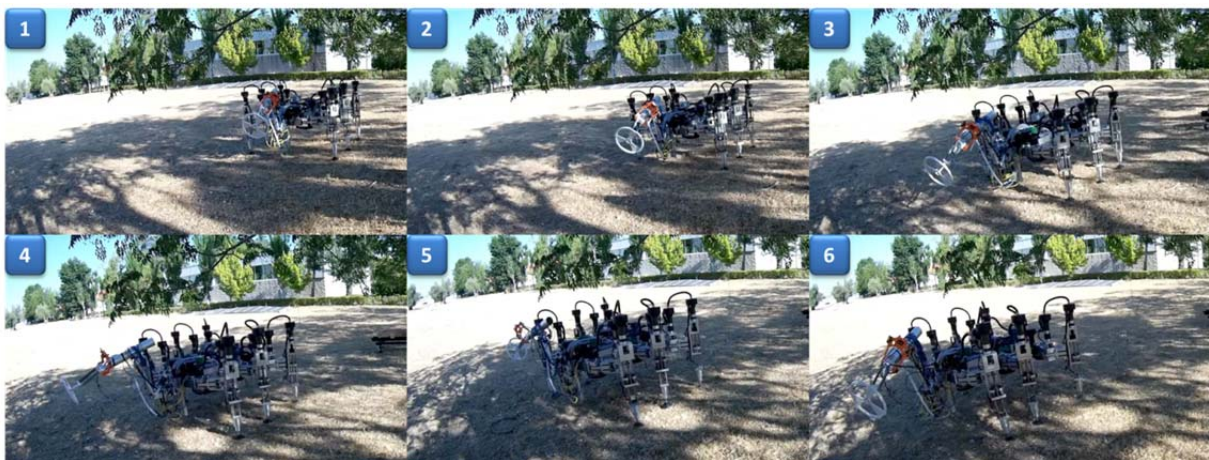
Figure 7. Photographic sequence of a continuous gait pattern of the hexapod robot.
