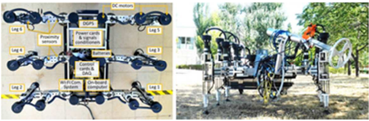
Figure 2. (a) Subsystems of the control architecture of the hexapod robot; (b) Hexapod walking robot at CSIC premises.
