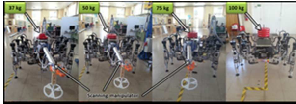
Figure 8. Photos with different loads put on the robot during the assessment of the energy consumption.
