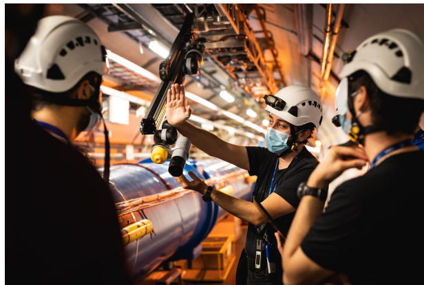
Figure 7.1: Train Inspection Monorail (TIM) platform for LHC tunnel operations, extensible with additional payloads such as a robotic arm (TIM Arm) [34].
