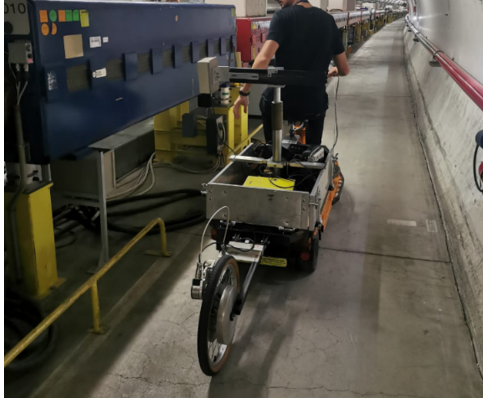
(a) Survey setup with measurement trolley and odometry wheel for distance tracking and data association.
