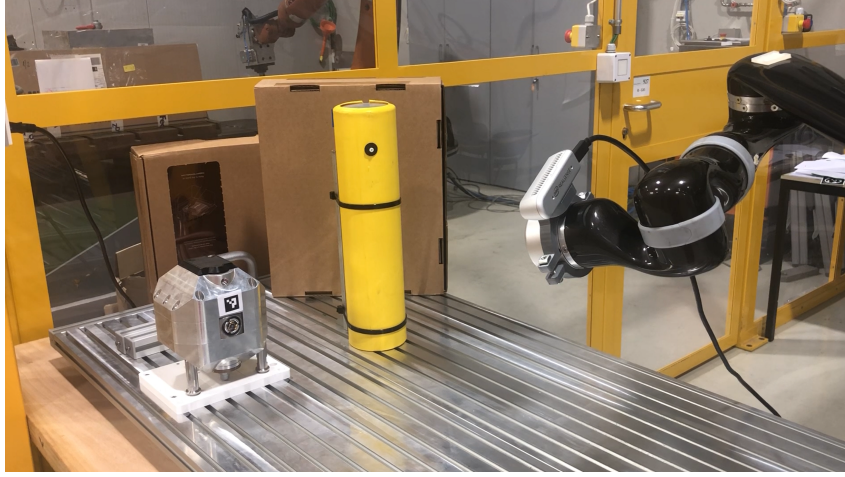
Figure 4.7: Experimental setup used for PBVS validation on the Kinova Gen2 arm. A fiducial marker is mounted on a fixed support, and an Intel RealSense camera is attached to the robot end-effector in an eye-in-hand configuration.
