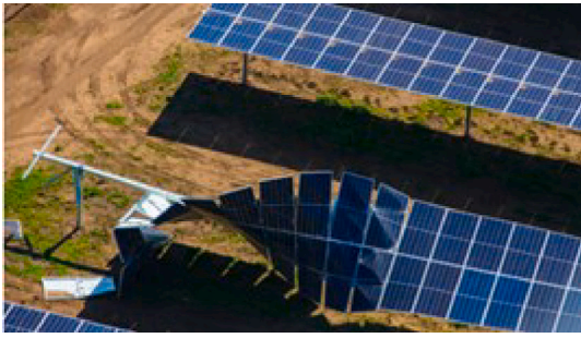
Fig. 3. Elements of an PST farm destroyed by wind-driven aeroelastic instability. Left: Oakey plant, Queensland, Australia (extracted from Gifford, 2019), right: Andalusia, Spain (extracted from Valentín et al., 2022).
