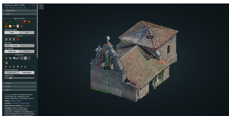
Figure 20. Results obtained after passing the 3D point cloud into the Potree viewer.
