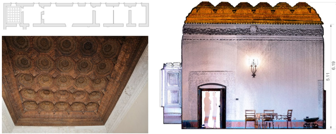
Figure 5. Corner room. Photograph, plan and section of the point cloud, by the authors. This room is covered by an alfarje, a horizontal ceiling. The geometric pattern is made up of octagons and squares.
