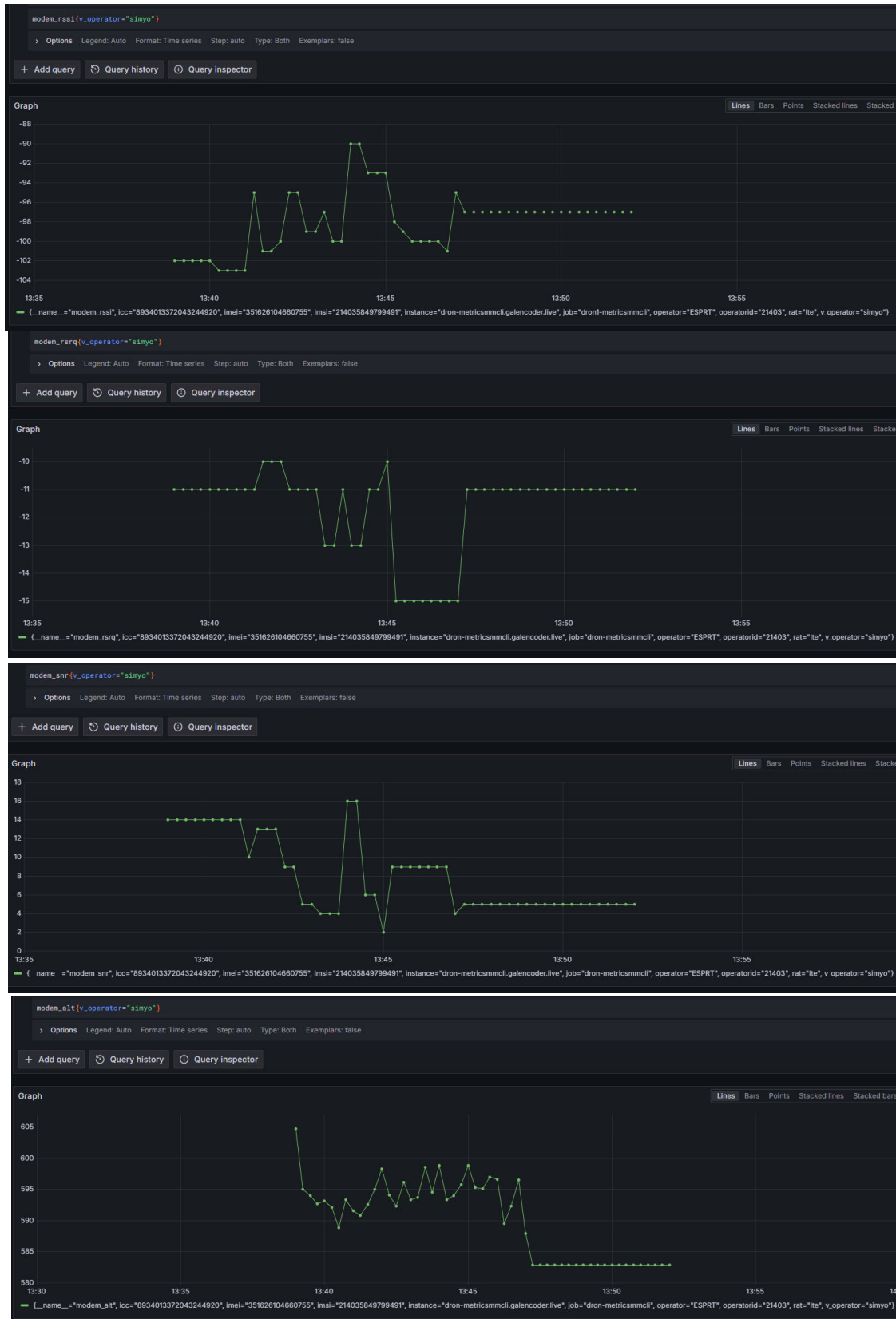
FIGURE 12. Collected Simyo data (RSSI, RSRQ, SNR, altitude) for an area around coordinates 41° 18'00.0"N 1° 39'36.0"W.
