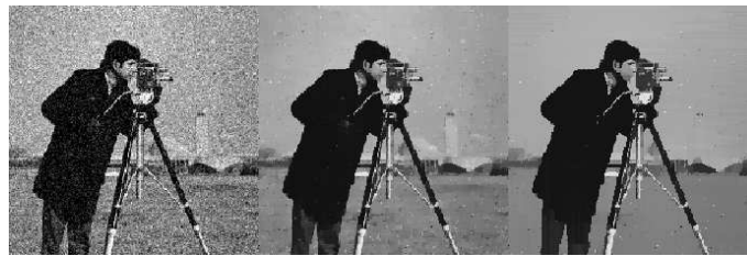
Figura 2. 2D filter with AOS a) Original, b) p = 2 , k = 1,8ms , c) p = 3 , k = 0,54ms
