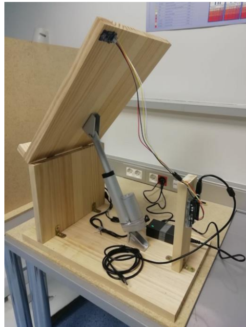
Figure 7. Experimental apparatus with the support of the samples completely inclined (50°).
