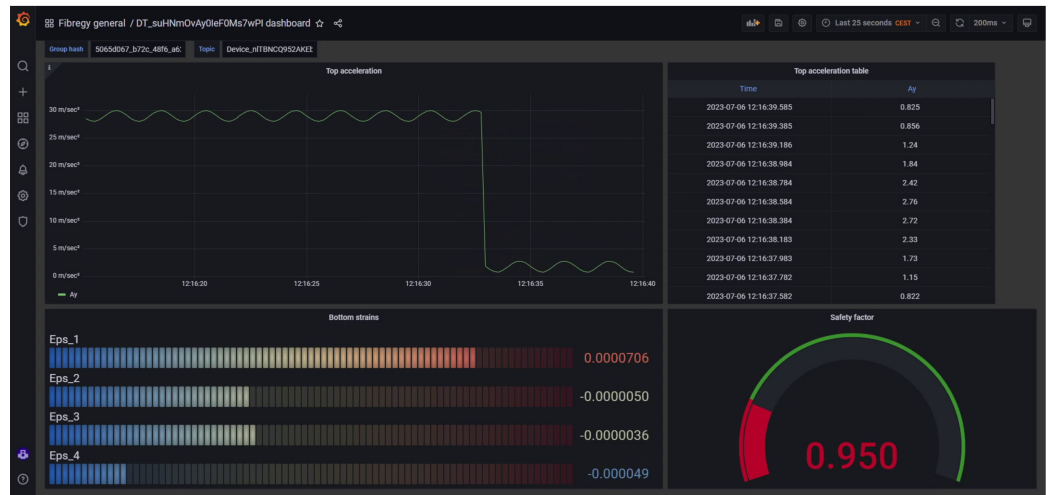
Figure 6. Real-time Grafana dashboard displaying structural and environmental signals, including strain, displacement, and wind data.
