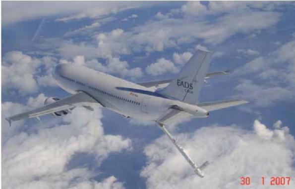
Fig. 2 Boom System in AIRBUS Military A310-Demo platform
