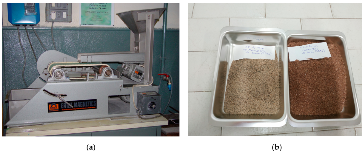
Figure 9. Separation by HIMS of the Santísima Trinidad sample. (a) Rare earth permanent magnet high-intensity magnetic separator and (b) fractions obtained from HIMS with rare earth permanent magnet at 0.5–1 mm (magnetic-siderite fraction, right vs. non-magnetic fraction, left).
