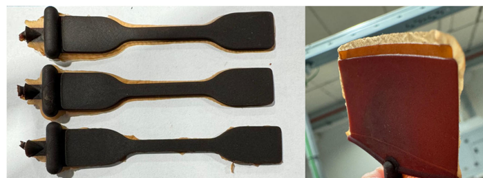
Figure 1. Visual comparison between dog-bones and squared plates of AES45.
