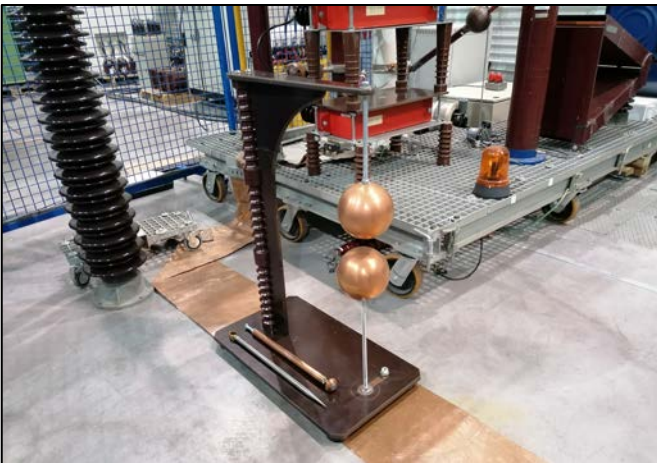
Fig. 7. Picture of the MV test cell for the quasi-homogeneous field.
