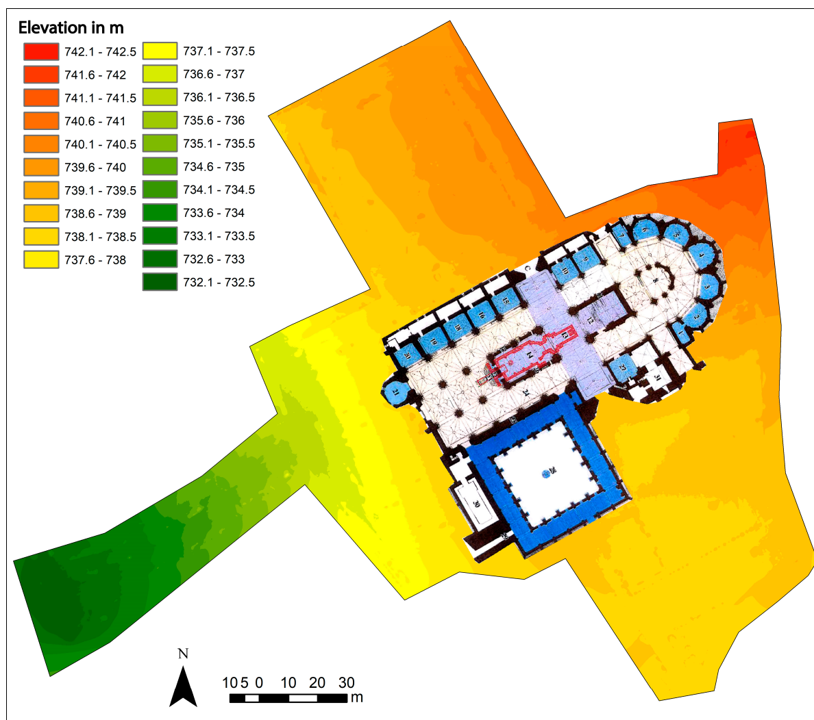
Figure 7. Hypsometric model (in meters) of the cathedral and neighboring areas. Note the terrain slope to the southwest, i.e., towards the Carrion River.
