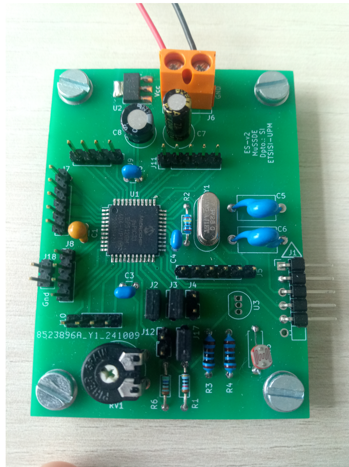
Figure 2. PCB with dsPIC33EP512GM604 used for developing and testing A \mu K.
