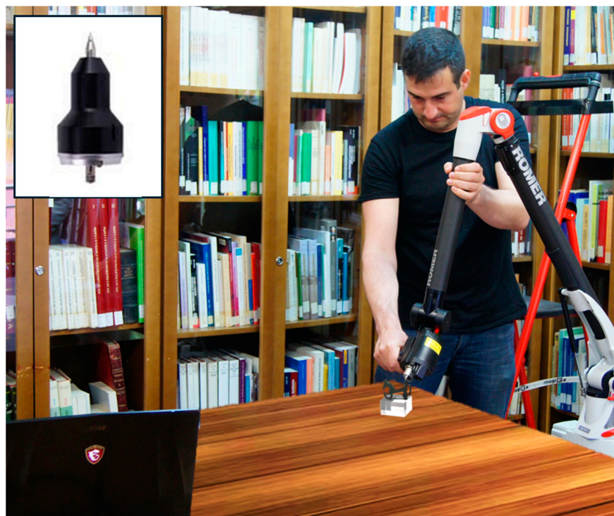
Figure 3. ACMM Hexagon Metrology Absolute Arm 7325SI employed for the ground truth.
