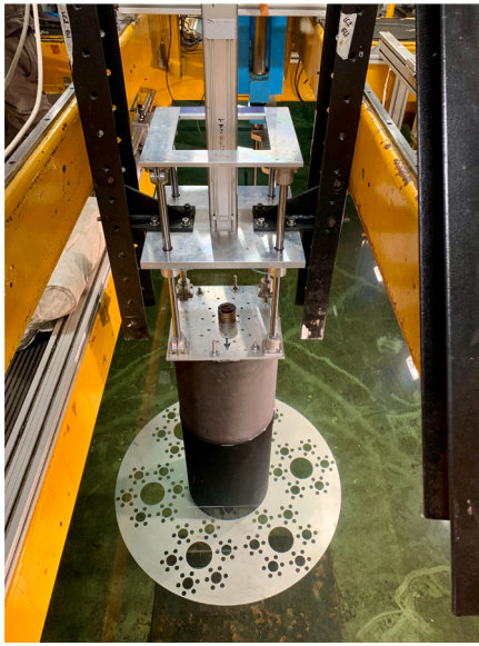
Fig. 1. Set up of the forced oscillation tests in ETSIN, UPM. The model is attached to the single DoF device.
