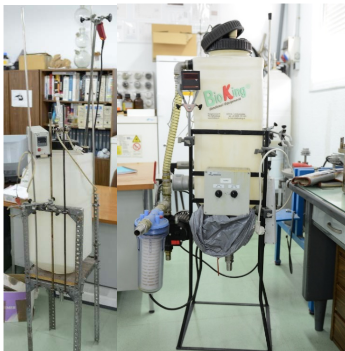
Figure. 7. 50 L reactors. On the left the one used for the wet wash, on the right the transesterification reactor.
