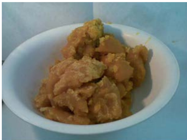
Fig. 22b. Graphical summary of the experimental troubles found in the production of FAME from castor oil: FAME from castor oil obtained with 2 % wt. of catalyst at 40 °C: the G-phase solidifies at room temperature due to the occurrence of soaps (5.3 % m/m).
