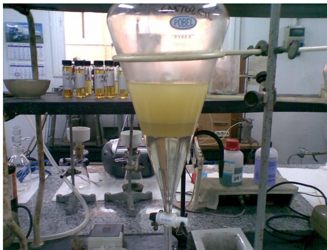
Figure 10. Graphical summary of the experimental troubles found in the production of FAME from castor oil: Irreversible emulsions formation in the “wet wash” purification method.
