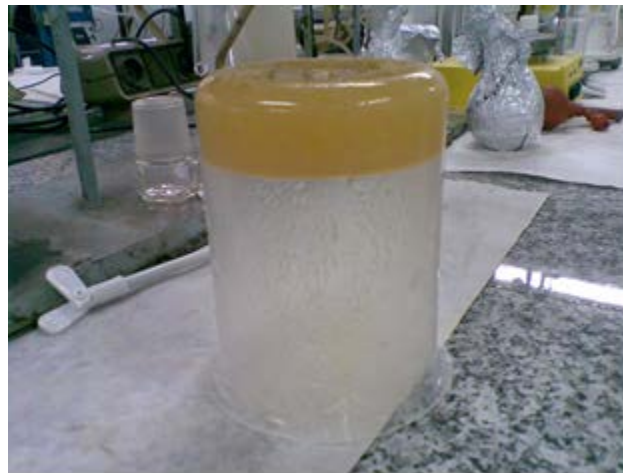
Fig. 22a. Graphical summary of the experimental troubles found in the production of FAME from castor oil: FAME from castor oil obtained at 60 °C: the FAME solidifies at room temperature due to the occurrence of soaps (3.7 % m/m)
