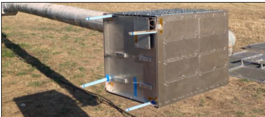
Figure 8. Radiation diagram measurement test using the STM
